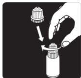
Pierce the BFS container by screwing the Two- parts Cap clock-wise.
